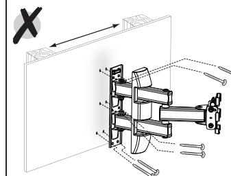
Using the provided self taping screws (B) type. Holding the TV mount starting in the one corner, screw the provided screws (B) into a wooden joist fixing the opposite corners, until the mount is secure onto the wall. Ensure all are tight and secure.
