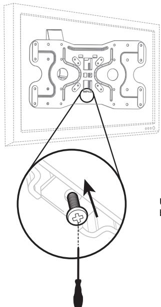
Using a screwdriver tighten the securing bolts onto the mount.
